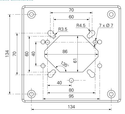
When the adapting plate is removed, the ModEva Pac attachment is mechanically compatible with DNC 880S
