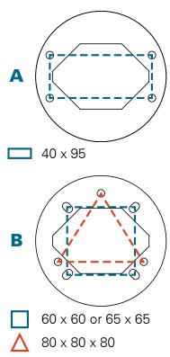
Two adapters are provided. Stick the appropriate one on top of the box.
